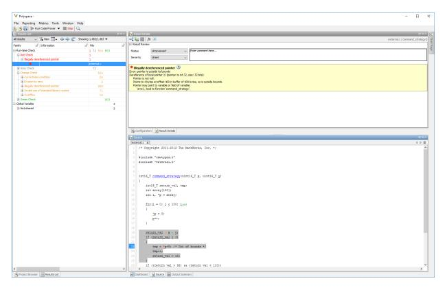
The Polyspace Code Prover error code indicates a problem with a pointer. Pointer \*p is out of bounds because it is used in an earlier loop. Correct the error by replacing this pointer with a variable of your choice, or deleting \*p from this line of code.
