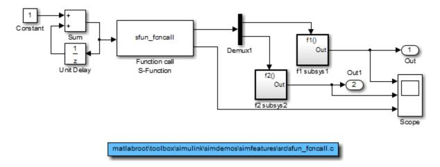
The first function-call subsystem provides a sine wave output. The second function-call subsystem is a simple feedback loop containing a Unit Delay block.
