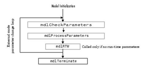
The engine calls mdlRTW once when it enters external mode and again each time a parameter changes or when you select **Simulation** > **Update Diagram**.
