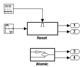
The model contains two nonvirtual subsystems, the conditionally executed enabled subsystem named Reset and the atomic subsystem named Atomic. Each subsystem contains an S-Function block that calls the S-function dsfunc.c, which models a discrete state-space system with two states. The enabled subsystem Reset resets the state values when the subsystem is enabled, and the output values when the subsystem is disabled.
