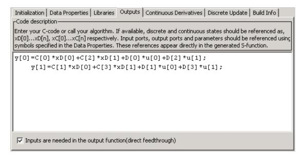
The **Outputs** pane also selects the **Inputs are needed in the output function (direct feedthrough)** option since this state-space model has a nonzero D matrix.
