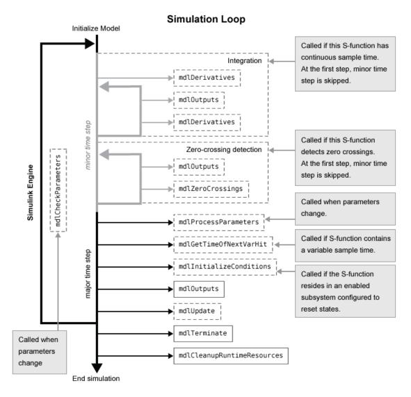
If your model contains multiple S-Function blocks at a given level of model hierarchy, the engine invokes a particular method for every S-function before proceeding to the next method. For example, the engine calls all the mdlInitializeSizes methods before calling any mdlInitializeSampleTimes methods. The engine uses the block sorted
