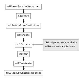
If the S-function resides in a conditionally executed subsystem, it is possible for the generated code to interleave calls to mdlInitializeConditions and mdlStart. Consider the following Simulink model sfcndemo enablesub.
