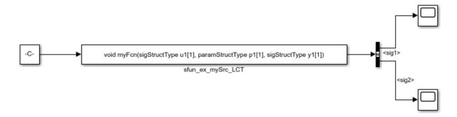
In the Constant block dialog box, the **Constant value** parameter is set to a structure whose fields match those of the structure type sigStructType. On the **Signal Attributes** tab, **Output data type** is set to the bus object sigStructType.
